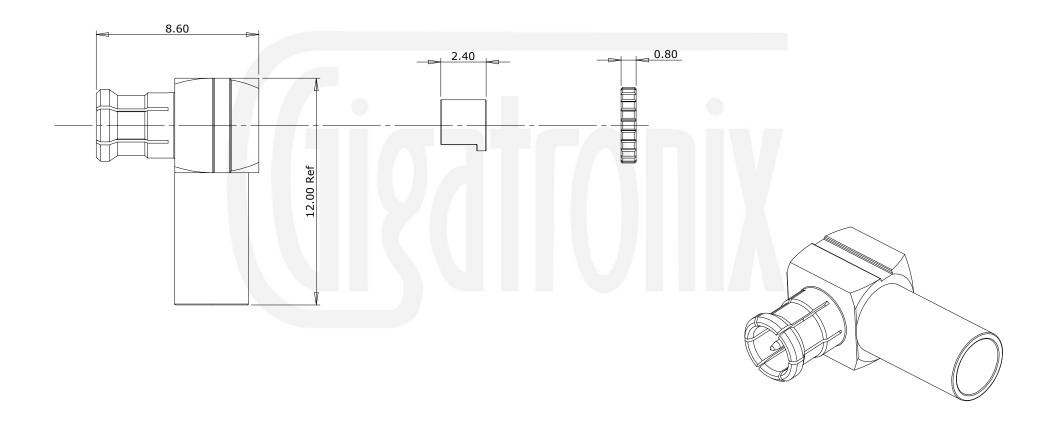
Unless otherwise specified tolerances  $0.5\text{-}5 = \pm 0.2$   $\Rightarrow 5\text{-}30 = \pm 0.4$   $\Rightarrow 30\text{-}120 = \pm 0.6$   $\Rightarrow 120\text{-}315 = \pm 1.0$   $\Rightarrow 315\text{-}1000 = \pm 1.6$  Angles =  $\pm 5^\circ$  Units = mm
